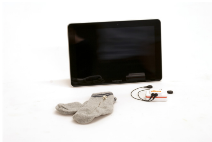
Fig. 4.08 Complete system(left) and integrated textile electrode (right)
