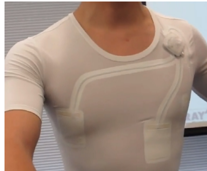
Fig. 4.03 Sensors embedded in sportswear
